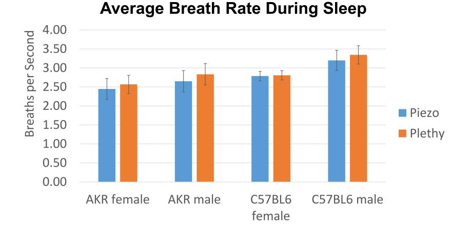
**Breath Rates calculated from piezoelectric sensor and** plethysmography during sleep. Percents shown are averaged from scored intervals of collective recordings of either male or female C57BL/6 or AKR mice.
